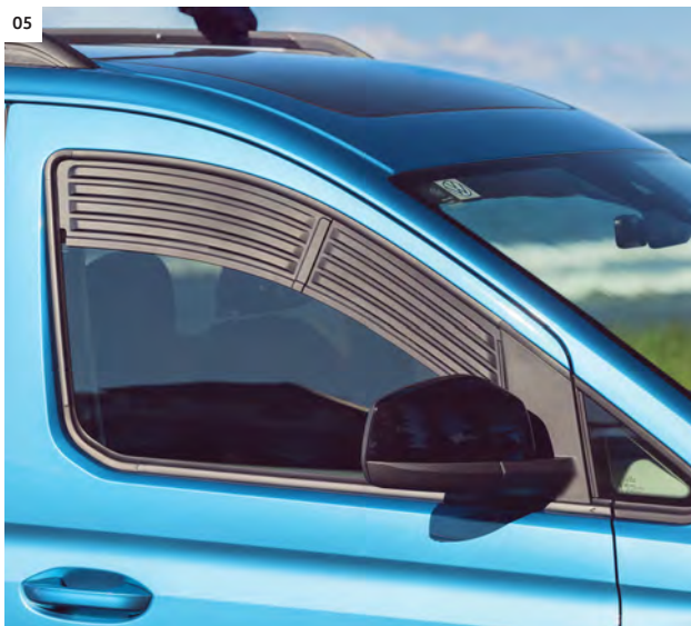
05 Two (2) ventilation grills with integrated fly screens.
