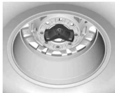
ZR2 Model Correctly Stored, Retainer Centered
