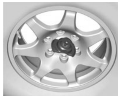
All Other Models Incorrectly Stored, Retainer Off-Center
