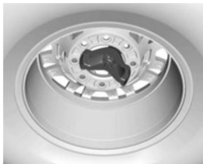
ZR2 Model Incorrectly Stored, Retainer Off-Center
