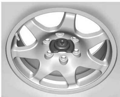
All Other Models Correctly Stored, Retainer Centered
