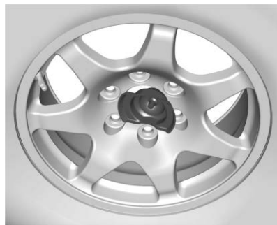
All Other Models Incorrectly Stored, Retainer Off-Center
