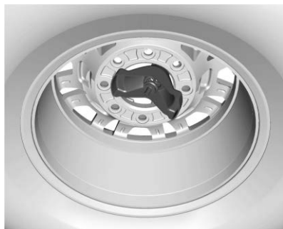
ZR2 Model Incorrectly Stored, Retainer Off-Center
