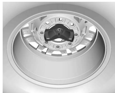
ZR2 Model Correctly Stored, Retainer Centered
