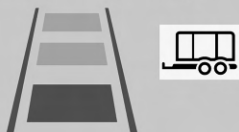
Near Gap Setting with Trailer
