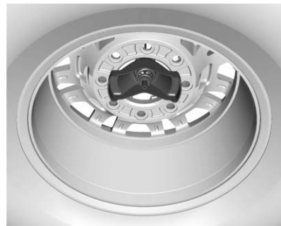
ZR2 Model Correctly Stored, Retainer Centered
