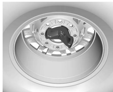
ZR2 Model Incorrectly Stored, Retainer Off-Center
